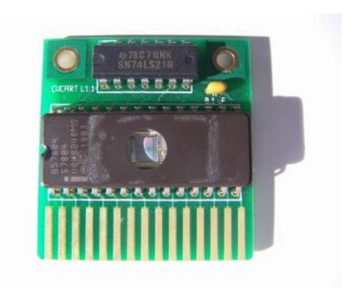
Figure 3: Incorrectly aligned EPROM
