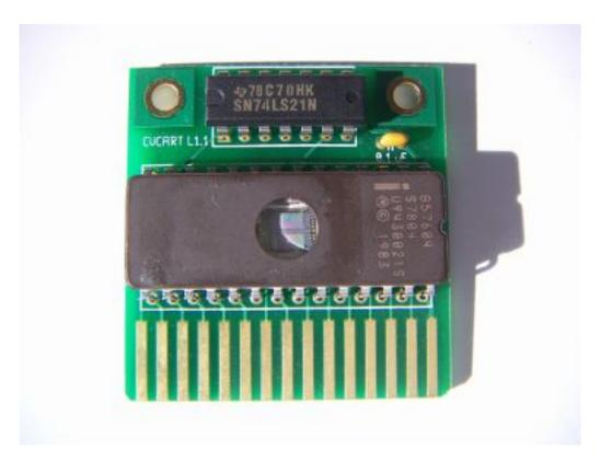
Figure 2: Correctly aligned EPROM and logic chip
