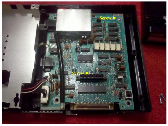
Remove the two screws shown above. You should now be able to remove the mainboard from the case. You'll also need to detach the power connector from the tray before removing. Pay attention to the orientation of the connector (wires facing down).
