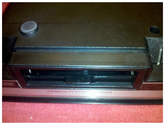
Turn the CV upside down. In the above image you will see that the tray is partially removed from the plastic expansion slot casing. While pulling backward on the tray, pull forward on the bottom of the bezel casing. This should expose the front edge of the tray. Work your way along to both ends of the bezel, exposing the rest of the tray. Once completed, the entire front edge of the tray should be exposed. You shouldn't have to lever the tray much from the back to make this happen.
