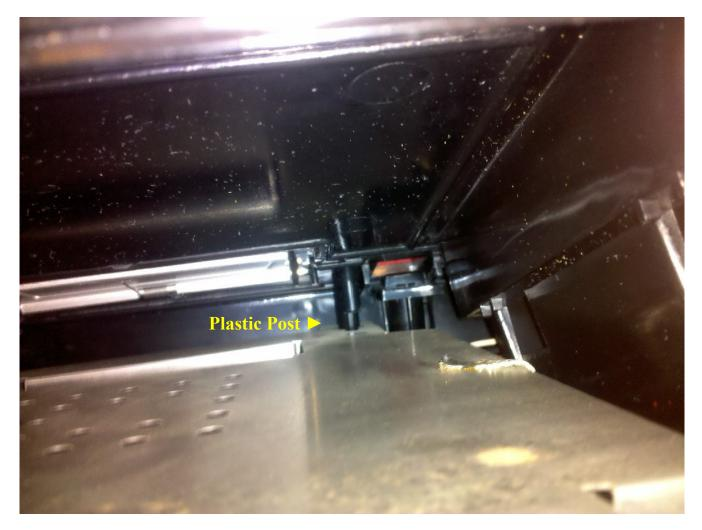
This plastic screw post, molded to the top and located next to the power switch, goes through a hole in the RF shield, and appears to keep the tray from being able to slide backwards more than  $\frac{1}{4}$  inch or so. However,  $\frac{1}{4}$  inch is all we need for the next step.
