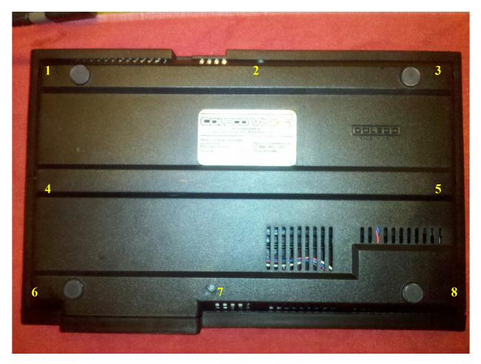
There are 8 screws on the bottom, numbered in the above image. Remove all of them with a phillips screwdriver and set them out of the way.
