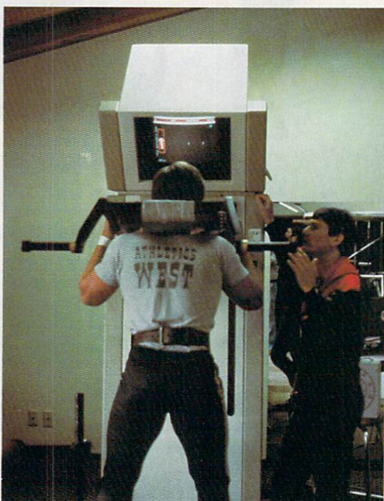
Top to bottom: A Coto Center staffer exercises while carefully watching the computer monitor; the graph on the screen displays the force of each up and down movement; an Olympic discus thrower practices the squat as a computer measures how much force he uses for each motion.
