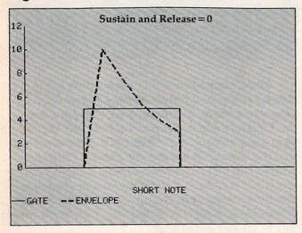
well. Figure 6 shows several combinations of attack, decay, and release values and how they interact with the gate to produce the sound envelope.
