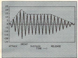
If you look at Figure 4, you will see how a sound looks if you could feed it into an oscilloscope. We can see the shape of the wave. The shape of the envelope defines the characteristics of a sound in a manner very similar to the way that harmonic content defines a sound.
