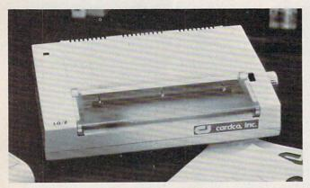
Cardco's LQ/2 is a \$349.95 letter-quality portable printer which prints 12 characters per second, and has built-in interfacing for all Commodore personal computers. It is also compatible with the PC, PCjr, TRS-80, and other computers with parallel Centronics printer output.
