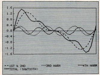
higher harmonics. You can see now that the resulting total waveshape is beginning to resemble a sawtooth, one of the waveforms available from the Commodore 64's Sound Interface Device (SID). If we kept adding the higher harmonics until we reached infinity, we would have a perfect sawtooth.
