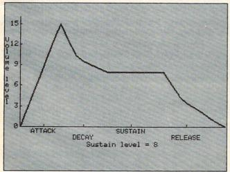
Not all sounds have this four-part volume envelope. Some have only an attack and release phase, and some (like the organ) have only the sustain phase. We can achieve all these on the Commodore 64 simply by setting the other phases to zero.
