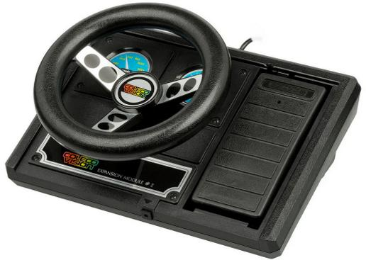
At its heart, the Driving Module comprises a steering wheel controller complete with an integrated gear shift and accelerator pedal. Through a dedicated port, the controller establishes a seamless line of communication with the ColecoVision console, translating the player's inputs into swift and precise actions within the game software.
