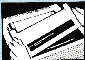
Remove the printer cover
