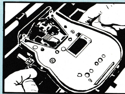
Press in the two latches located on either side of print mechanism
