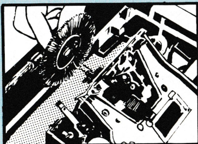
Place a new daisy wheel on the spindle
