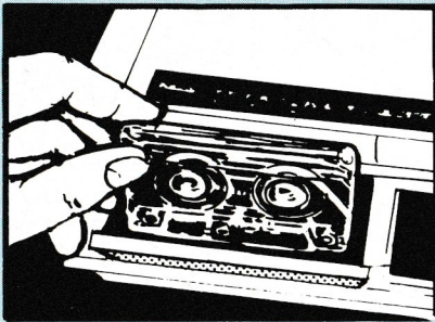
Insert the digital data pack into the digital data pack drive
