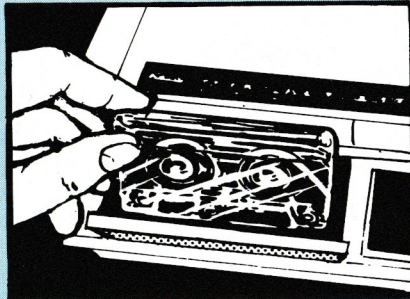
Insert or remove the digital data pack
