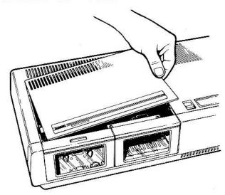
Step 1. Remove the top cover of your ADAM Memory Console by sliding your finger or the blade of a screwdriver in the indentation on the right and lifting up.
