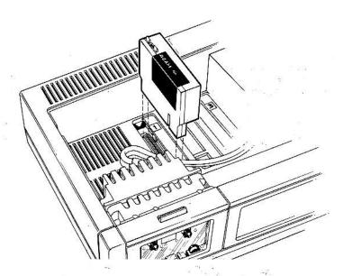
Step 2. Look inside the Memory Console. There are three expansion ports. These expansion ports are labeled 1, 2, and 3 on the plastic casing to their right.
